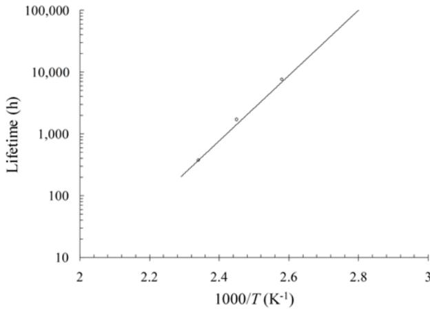
Fig. 6. Mineral oil lifetime line for  $M_T$  method.
