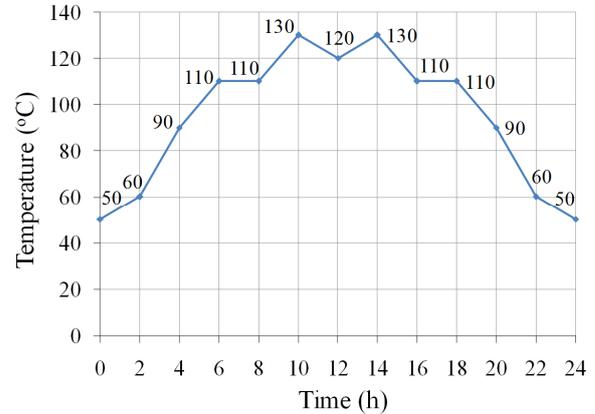
Fig. 7. Variation of the transformer insulation temperature ( $T$ ) with time – first version.
