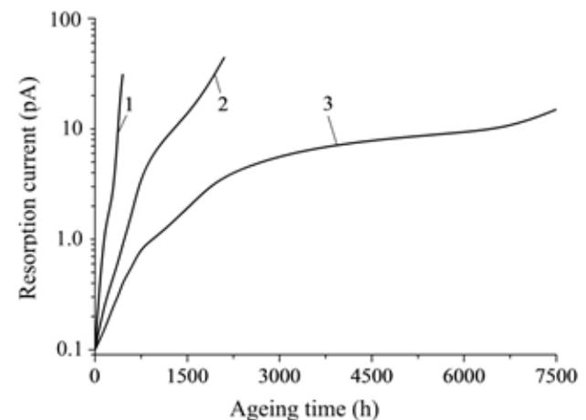
Fig. 4. Resorption currents variation with oil ageing time at 155 °C (1), 135 °C (2) and 115 °C (3).
