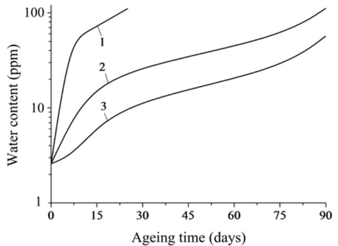
Fig. 2. The variation of water content in oil with ageing time at 155 °C (1), 135 °C (2) and 115 °C (3).
