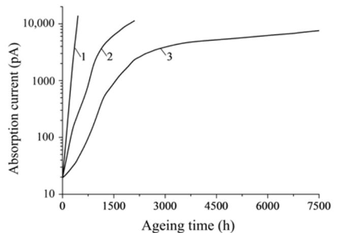
Fig. 3. Absorption currents variation with oil ageing time at 155 °C (1), 135 °C (2) and 115 °C (3).
