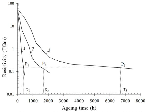
Fig. 5. Resistivity variation with oil ageing time at 155 °C (1), 135 °C (2) and 115 °C (3).
