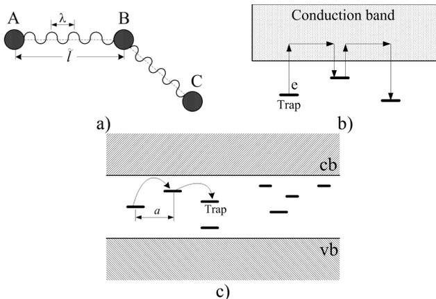
Fig. 1. Electron transport: a) Nearly free electrons in conduction band; b) Trap-controlled band transport; c) Hopping transport (A, B, C – scattering centers,  $\lambda$  – de Broglie wavelength,  $l$  – mean free path,  $e$  – electron,  $cb$  – conduction band and  $vb$  – valence band).
