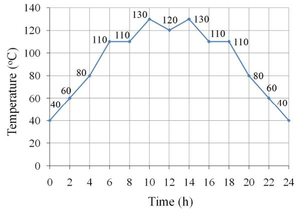
Fig. 8. Variation of the transformer insulation temperature ( $T$ ) with time – second version.
