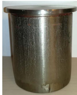
Figure 3. Stainless steel cell for samples thermal aging
